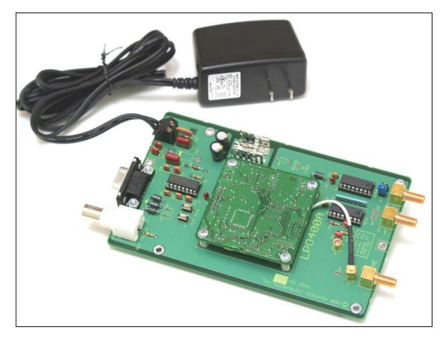
The LPO400A evaluation board is similar to the 440A, but is supplied without a case to make evaluation of the LPO400A module easier. See the board parts placement diagram and schematic below for details on the evaluation board.
